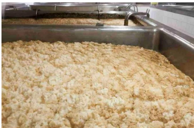
Figure 1: An Industrial beer brewing set up showing Krausen, the head formed at the peak of fermentation.
